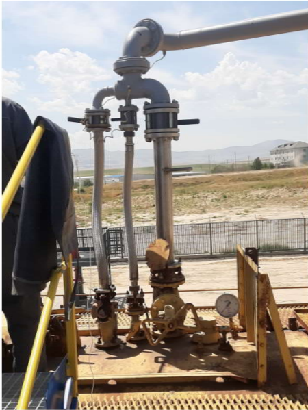
Coaxial loading arm for liquefied gas hermetic loading under pressure
