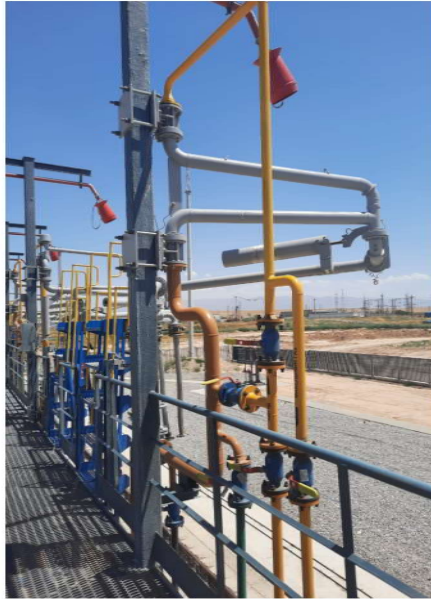
Coaxial loading arm for liquefied gas hermetic loading under pressure
